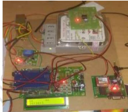
Figure 1. GSM Based Smart Energy Meter with Arduino Uno
