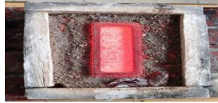
Figure 4. Microwave casting experimentation with specimen
