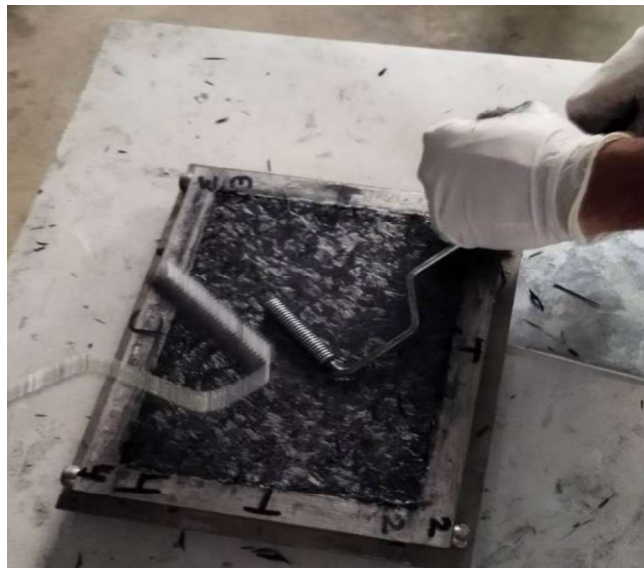
Fig. 3 Fabrication of Chopped CFREC
