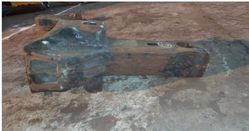
Fig. 8 Casted coupler after finishing and machined
