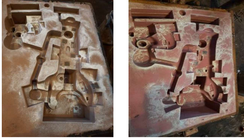
Fig. 7 Cope and drag prepared with sand prepared for coupler casting.
