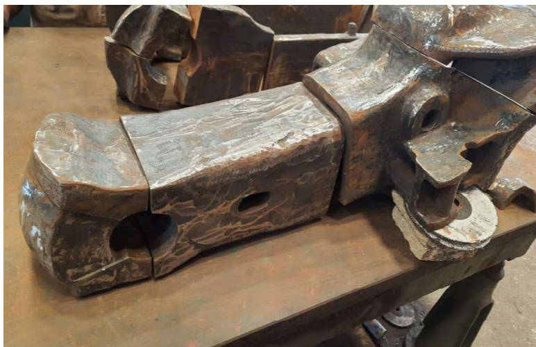
Fig. 10 Location of the cut sections for inspection as per RDSO specification
