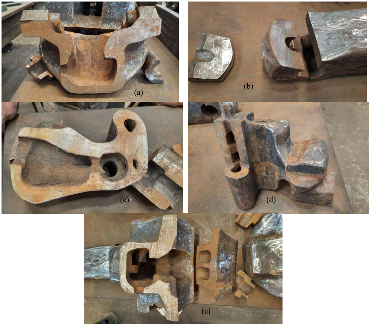
Fig.11 Details of the cut sections of the 70 BD coupler for inspection
